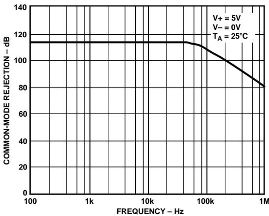
TPC 17. Common-Mode Rejection vs. Frequency @ 5 V
