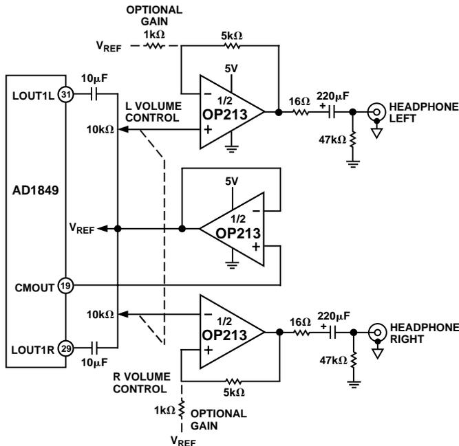
Figure 9. Headphone Output Amplifier for Multimedia Sound Codec
