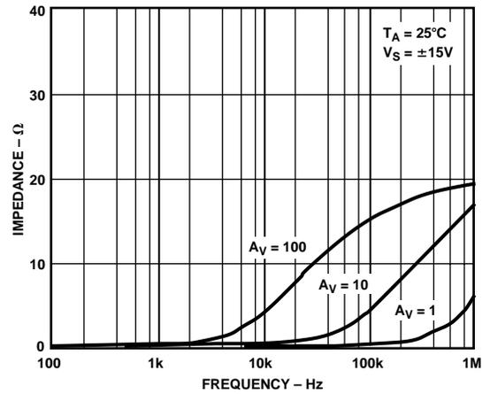
TPC 24. Closed-Loop Output Impedance vs. Frequency @ ±15 V
