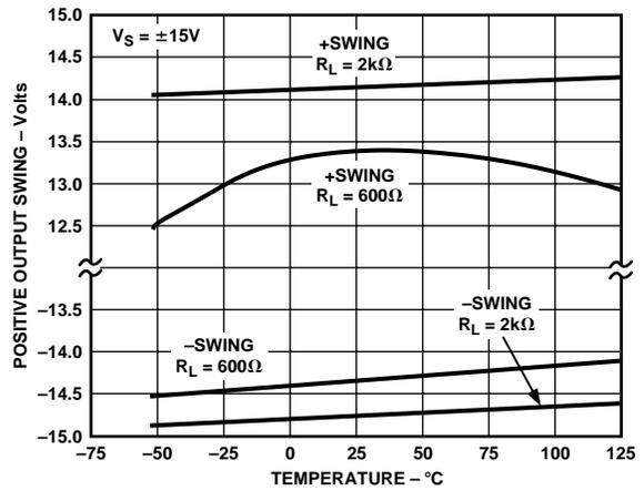
TPC 7. Output Swing vs. Temperature and  $R_L$  @ ±15 V
