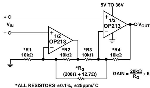
Figure 5. Ultralow Noise, Single Supply Instrumentation Amplifier
