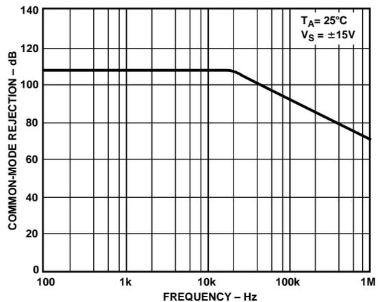
TPC 20. Common-Mode Rejection vs. Frequency @ ±15 V
