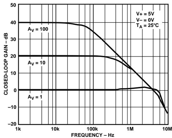
TPC 11. Closed-Loop Gain vs. Frequency @ 5 V
