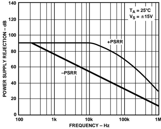
TPC 21. Power Supply Rejection vs. Frequency @ ±15 V
