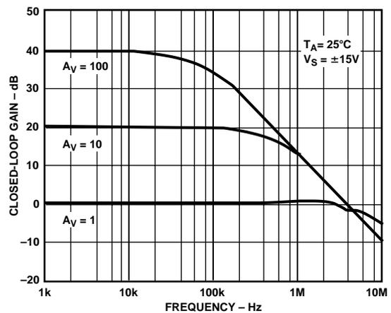
TPC 14. Closed-Loop Gain vs. Frequency @ ±15 V
