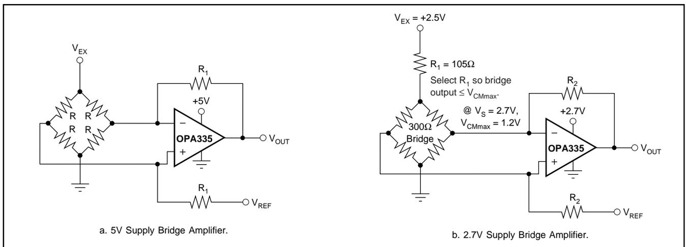
FIGURE 5. Single Op Amp Bridge Amplifier Circuits.
