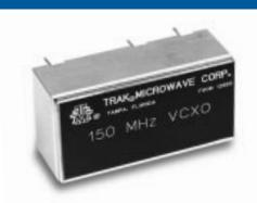
This miniature ovenized VCXO utilizes a specially mounted AT-cut crystal which helps determine the unit's excellent spurious and low vibration sensitivity levels. This unit is practically spur free at offsets under 45 kHz and has typical vibration sensitivity as low as  $2.5 \times 10^{-9}$ /g.
