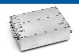
This PLDRO uses two phase lock loops for good phase noise performance. The 6.6 GHz DRO, which drives the far-out noise levels, is phase locked to an internal 110 MHz PLXO, which drives the moderately close-in noise; close-in noise is a function of the phased locked PLXO and input 5 MHz reference.
