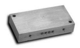
This model is a thin-film, hybrid microelectronics Phase Locked Oscillator housed in a hermetically sealed Kovar housing. The circuitry is printed on three alumina substrates loaded with active dies, tantalum nitride resistors and ceramic capacitors. Interconnections are made using a combination of wedge and ball bonded gold wires and internal feedthroughs.
