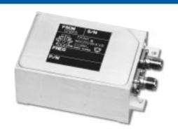
This hermetically sealed phase locked DRO uses MIC thin-film construction to provide a very small package size without compromising output spectral purity. The unit is based on a bipolar transistor oscillator and boasts a + 16 dBm RF output level.
