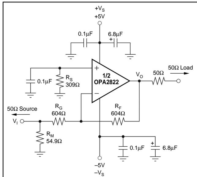
FIGURE 2. Inverting  $G = -1$  Specifications and Test Circuit.
