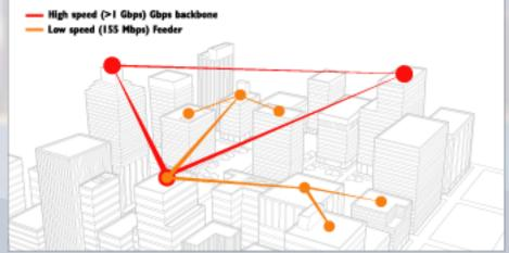
"OptiBridge<sup>TM</sup> 2500 is the first commercially available, single channel, free-space optical transceiver that delivers 2.5 Gbps over 2 km."
