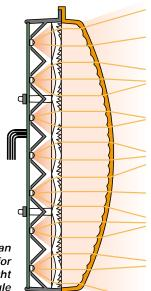
Schematic view of an optical system for the OSRAM OS traffic light module
