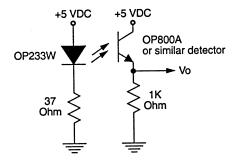
Replacement pulsed drive current circuit:
