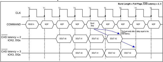
If a Burst Stop Command is issued during a full page burst write operation, then any residual data from the burst write cycle will be ignored. Data that is presented on the DQ pins before the Burst Stop Command is registered will be written to the memory.
