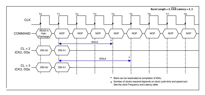
Similar to the Read Command, a Write Command with auto-precharge can not be interrupted by a command to the same bank. It can be interrupted by a Read or Write Command to a different bank, however. The precharge function will begin with the new command. The bank may be reactivated after tRP is satisfied.
