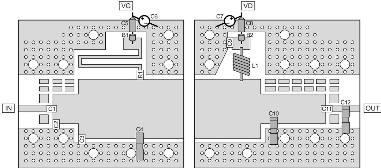
TEST CIRCUIT SCHEMATIC FOR 850 TO 900 MHz
