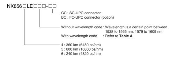
Table A: DWDM wavelengths based on ITU-T recommendations (@TLD = Tset) (1/2)
