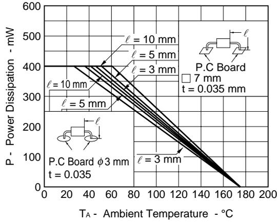
Fig. 2 THERMAL RESISTANCE vs. SIZE OF P.C BOARD
