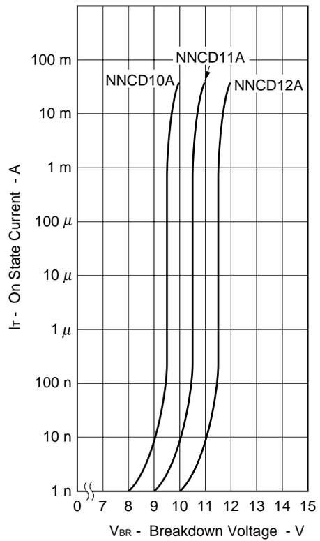
Fig. 5  $Z_z - I_T$  CHARACTERISTICS
