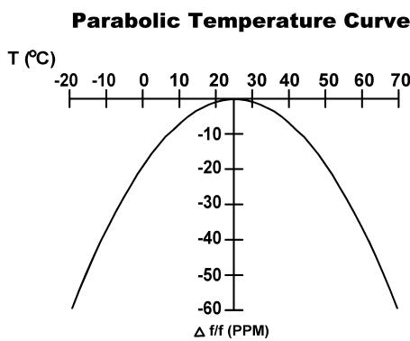
To determine frequency stability, use parabolic curvature (K).
