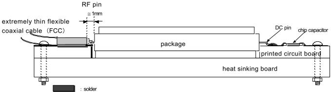
Caution: The package base should be connected to the ground.
