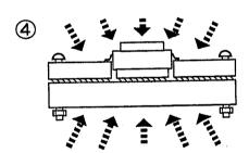
Again fasten the printed circuit board to the heat sinking board with the screws. Bake the fixture in an oven for 60 minutes at  $150^{\circ}$  ( $120^{\circ}$   $\sim$   $170^{\circ}$ ).
