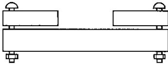
Temporarily fasten the printed circuit board to the heat sinking board with the screws.
