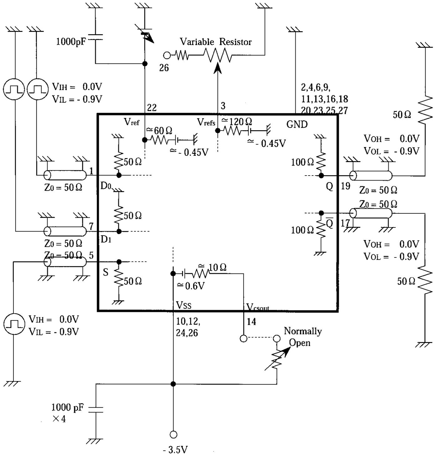
As shown above, two methods exist for applying a DC voltage to the  $V_{ref}$  and  $V_{refs}$  pins. One involves a voltage divider using a variable resistor, while in the other, an external power supply is connected directly. Apply approximately  $-0.5V$  to each pin in the latter case.
