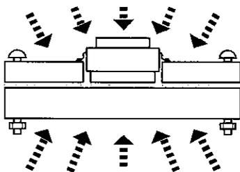
Again fasten the printed circuit board to the heat sinking board with the screws. Bake the fixture in an oven for 60 minutes at 150°C (120°C~170°C).
