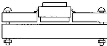
Insert the IC package into the center part of the printed circuit board. Solder the GND pins to the printed circuit board.
