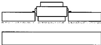
Unfasten the printed circuit board from the heat sinking board. Thinly paint the entire bottom surfaces of the printed circuit board and the IC with the conducting epoxy adhesive. Make sure that silver paste is not applied to the region between the printed circuit board and the IC.
