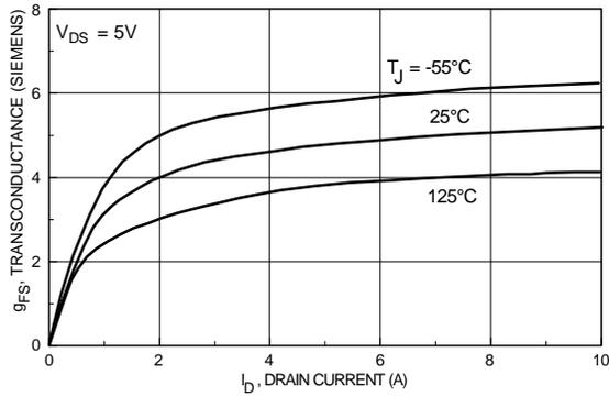
Figure 13. Transconductance Variation with Drain Current and Temperature.
