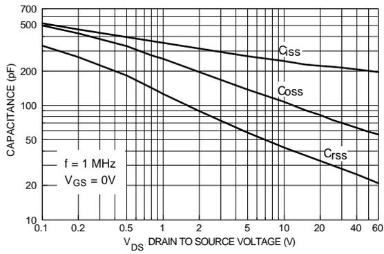
Figure 9. Capacitance Characteristics.
