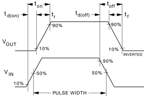
Figure 12. Switching Waveforms.
