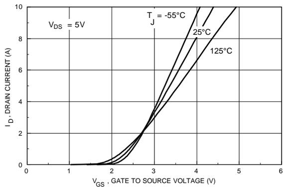
Figure 5. Transfer Characteristics.
