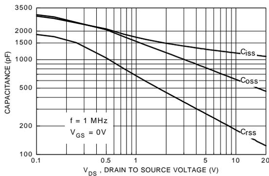
**Figure 9. Capacitance Characteristics.**
