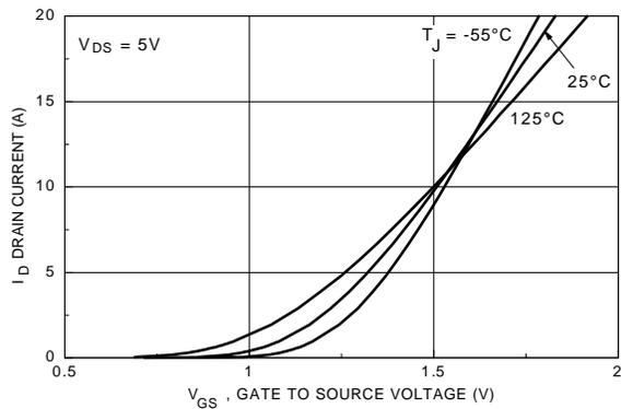
Figure 5. Transfer Characteristics.
