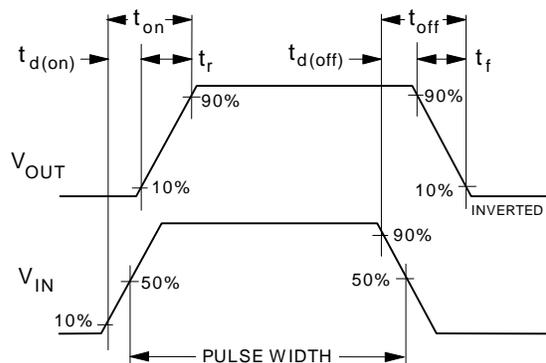
**Figure 12. Switching Waveforms.**
