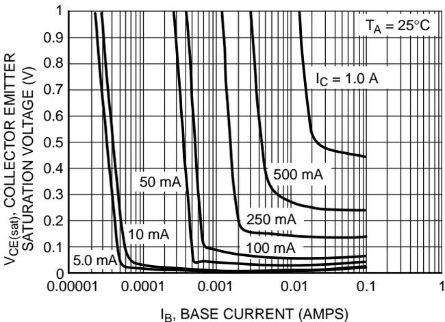
Figure 5. Collector Emitter Saturation Voltage vs Base Current
