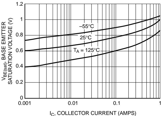
Figure 6. Base Emitter Saturation Voltage vs. Collector Current
