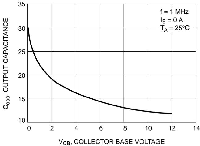
**Figure 9. Output Capacitance**
