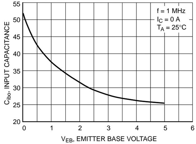
**Figure 8. Input Capacitance**
