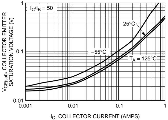
Figure 4. Collector Emitter Saturation Voltage vs. Collector Current
