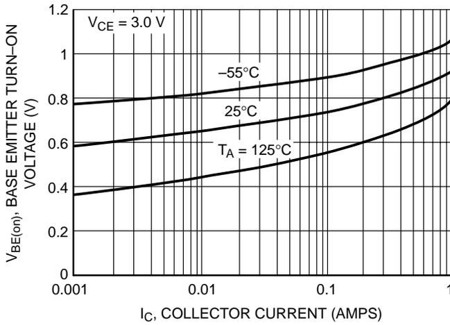
**Figure 7. Base Emitter Turn-On Voltage vs. Collector Current**
