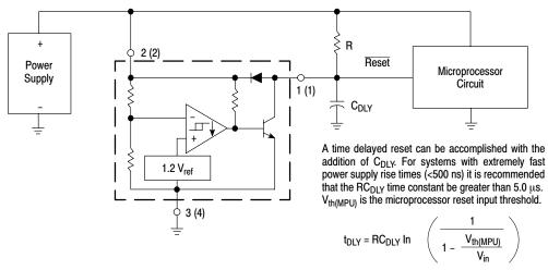
Figure 9. Low Voltage Microprocessor Reset
