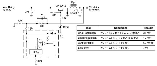
Figure 13. Low Power Switching Regulator
