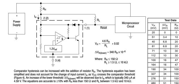
Figure 10. Low Voltage Microprocessor Reset with Additional Hysteresis
