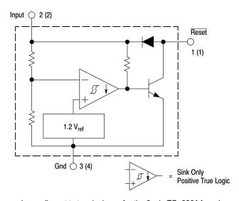
Pin numbers adjacent to terminals are for the 3–pin TO–226AA package. Pin numbers in parenthesis are for the 8–lead packages.
