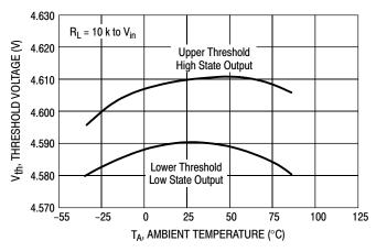
Figure 4. Comparator Threshold Voltage versus Temperature
