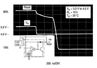
Figure 7. Reset Delay Time
