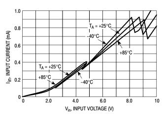
Figure 5. Input Current versus Input Voltage
