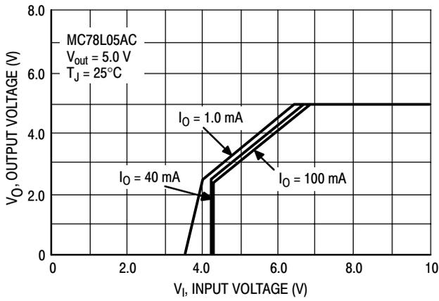
Figure 3. Dropout Characteristics
