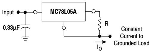
The MC78L00 regulators can also be used as a current source when connected as above. In order to minimize dissipation the MC78L05C is chosen in this application. Resistor R determines the current as follows:
