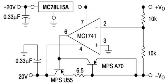
Figure 10. ± 15 V Tracking Voltage Regulator
