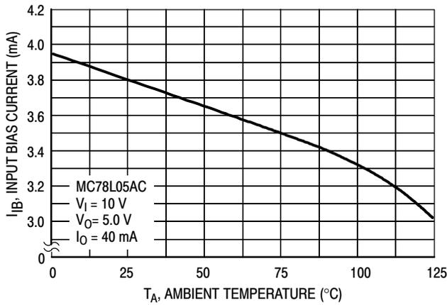
Figure 5. Input Bias Current versus Ambient Temperature
