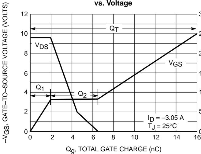
**Figure 9. Gate-to-Source and Drain-to-Source Voltage vs. Total Charge**
