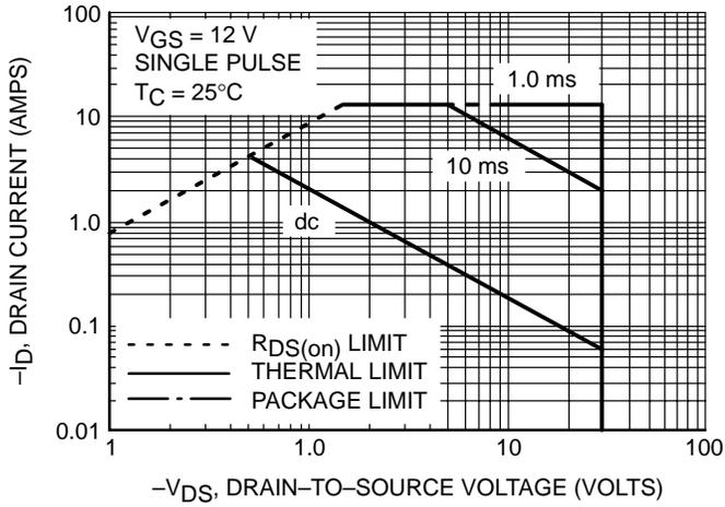
**Figure 13. Maximum Rated Forward Biased Safe Operating Area**
