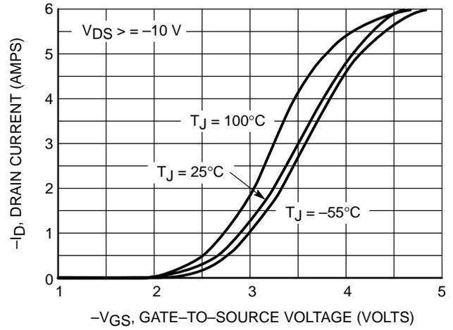
Figure 2. Transfer Characteristics
