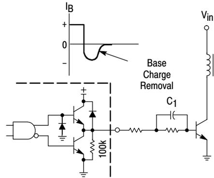
The totem-pole outputs can furnish negative base current for enhanced transistor turn-off, with the addition of capacitor C1.
