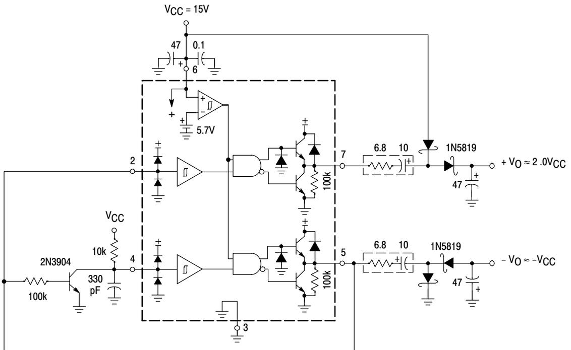
The capacitor's equivalent series resistance limits the Drive Output Current to 1.5 A. An additional series resistor may be required when using tantalum or other low ESR capacitors.
