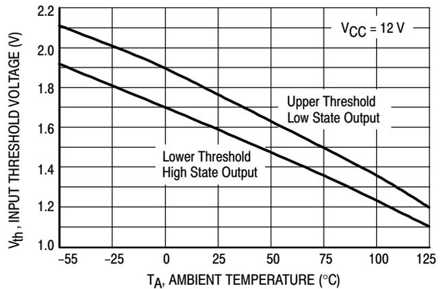
Figure 5. Logic Input Threshold Voltage versus Temperature
