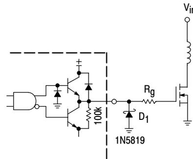
Series gate resistor  $R_g$  may be needed to damp high frequency parasitic oscillations caused by the MOSFET input capacitance and any series wiring inductance in the gate-source circuit.  $R_g$  will decrease the MOSFET switching speed. Schottky diode  $D_1$  can reduce the driver's power dissipation due to excessive ringing, by preventing the output pin from being driven below ground.
