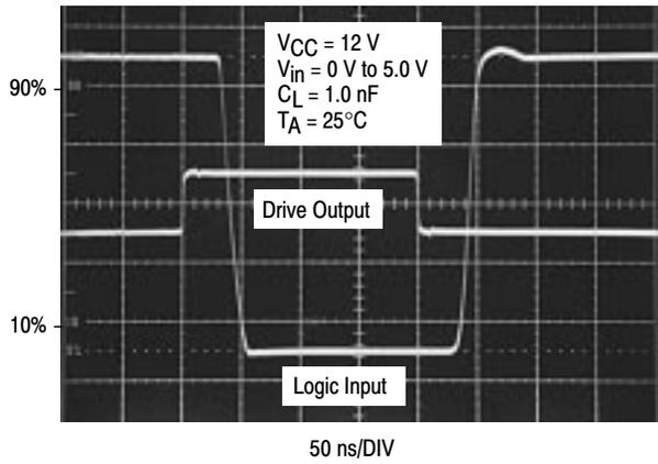
Figure 8. Propagation Delay
