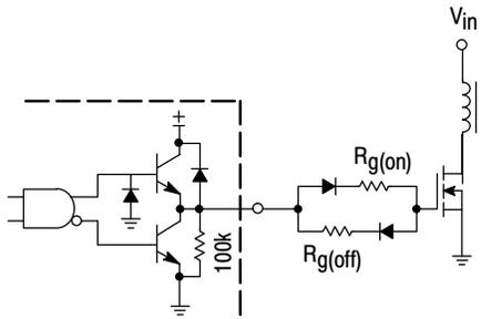
In noise sensitive applications, both conducted and radiated EMI can be reduced significantly by controlling the MOSFET's turn-on and turn-off times.
