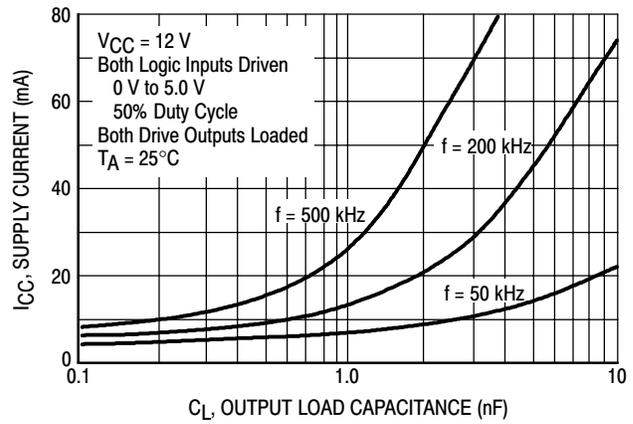
**Figure 15. Supply Current versus Drive Output Load Capacitance**
