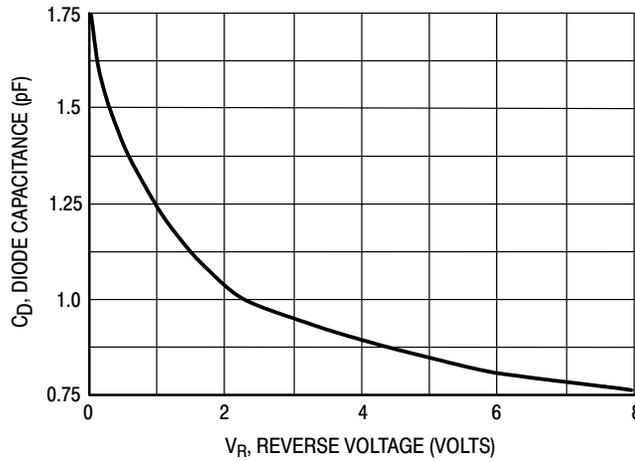
Figure 3. Diode Capacitance
