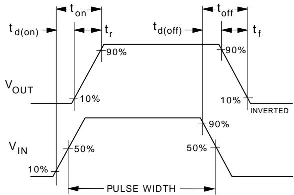
Figure 12. Switching Waveforms.
