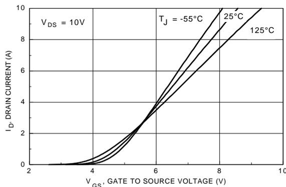
Figure 5. Transfer Characteristics.
