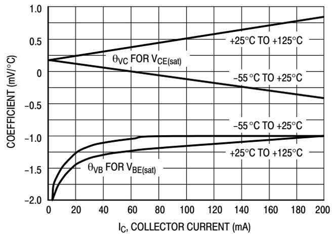
Figure 17. Temperature Coefficients
