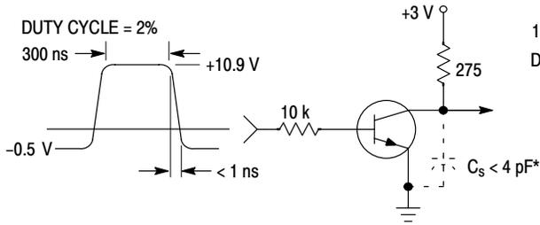
**Figure 1. Delay and Rise Time Equivalent Test Circuit**
