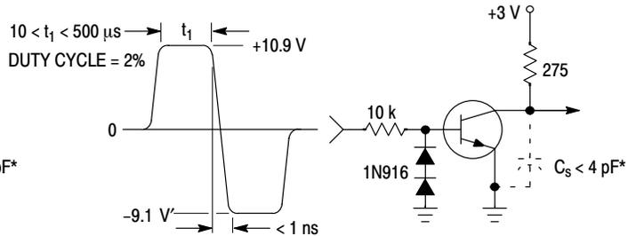
**Figure 2. Storage and Fall Time Equivalent Test Circuit**
