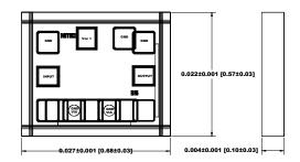
**<u>Electrical Specifications</u>**  $V_{cc1}$ = +10V,  $V_{cc2}$ = +10V,  $V_{c1}$ =+4.75 V,  $V_{c2}$ = +2.98V,  $I_{cc2}$  = 40 mA, Zo = 50Ω,  $T_A$  = +25 °C
