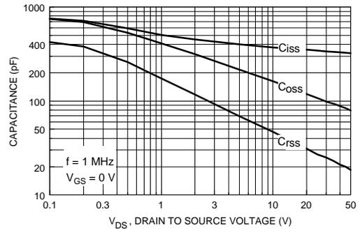
Figure 8. Capacitance Characteristics.
