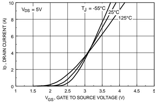
Figure 5 . Transfer Characteristics.
