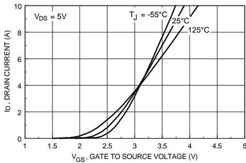
Figure 5. Transfer Characteristics.
