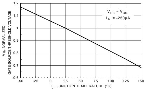
**Figure 12.** P-Channel Gate Threshold Variation with Temperature.
