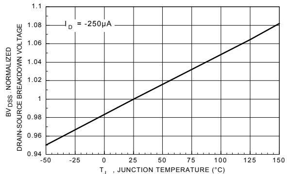
**Figure 14.** P-Channel Breakdown Voltage Variation with Temperature.
