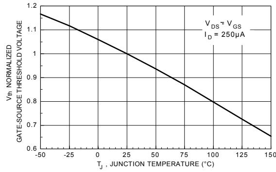
**Figure 11.** N-Channel Gate Threshold Variation with Temperature.
