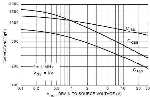
**Figure 15.** N-Channel Capacitance Characteristics.
