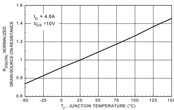
**Figure 5. N-Channel On-Resistance Variation with Temperature.**
