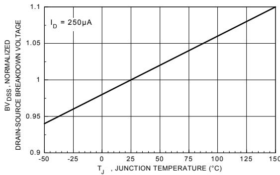
**Figure 13.** N-Channel Breakdown Voltage Variation with Temperature.
