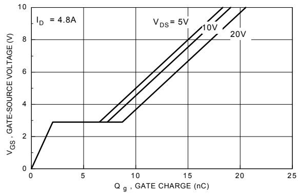
**Figure 17.** N-Channel Gate Charge Characteristics.
