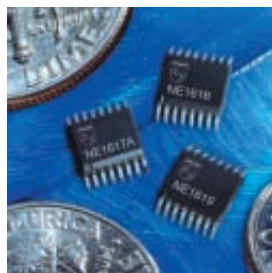
Philips sensors operate at a temp range of 0 to +120°C
