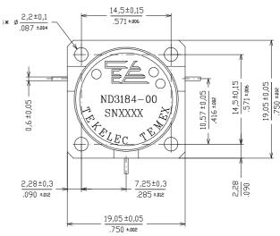
Housing: Steel Housing finish: Nickel Contact material: CuBe2 Contact finish: silver
