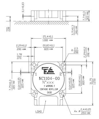
Housing finish: Nickel Contact material: CuBe2 Contact finish: silver
