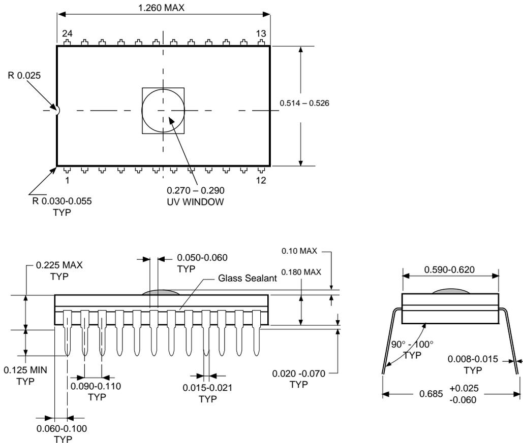
**UV Window Cavity Dual-In-Line Package (Q)**
