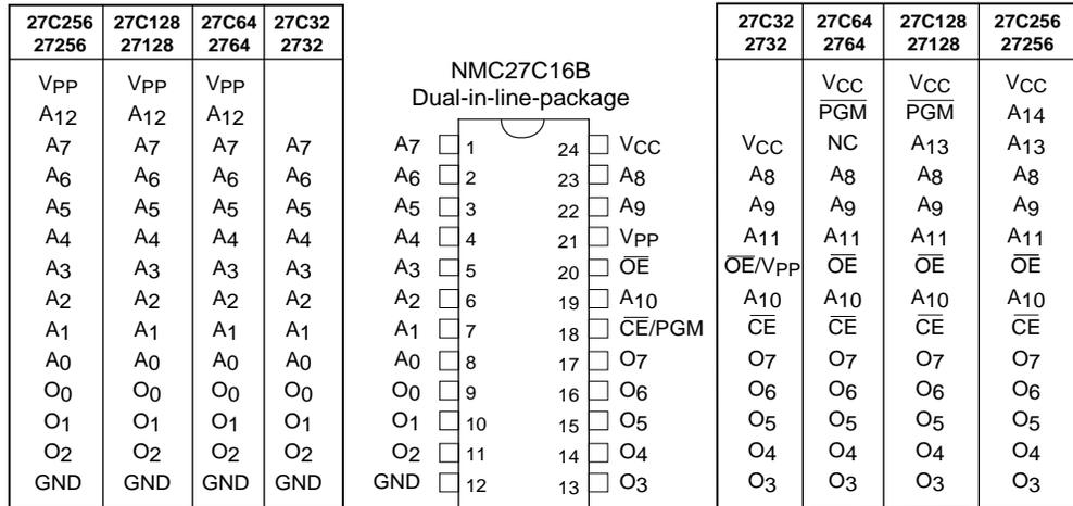
**Note:** Socket compatible EPROM pin configurations are shown in the blocks adjacent to the NMC27C16B pins.
