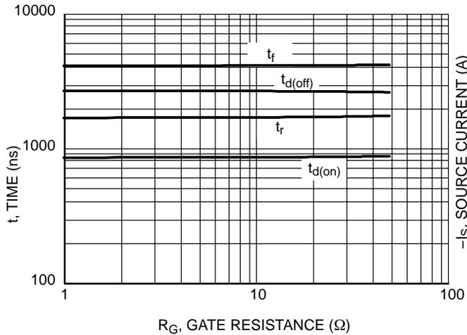
**Figure 9. Resistive Switching Time Variation Gate Resistance**
