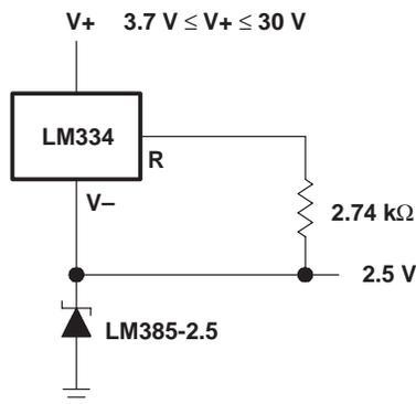
Figure 11. Operation Over a Wide Supply Range
