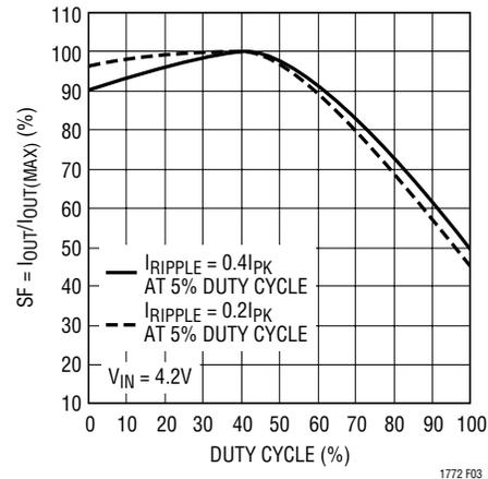
Figure 3. Maximum Output Current vs Duty Cycle
