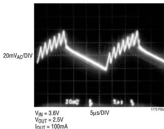
**$V_{OUT}$  Ripple for Figure 1 Circuit Using LTC1772B Non-Burst Mode Operation.**
