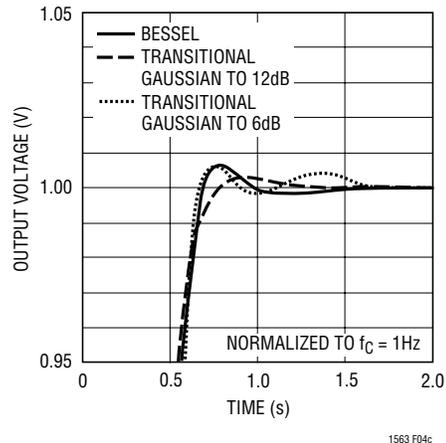
Figure 6c. Step Response—Settling
