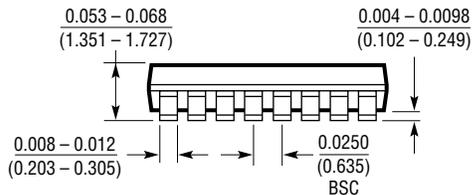
\* DIMENSION DOES NOT INCLUDE MOLD FLASH. MOLD FLASH SHALL NOT EXCEED 0.006" (0.152mm) PER SIDE
