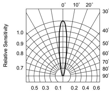
FIG.5 SENSITIVITY DIAGRAM
