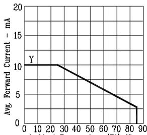
Fig5. MAX. AVERAGE FORWARD CURRENT VS. AMBIENT TEMPERATURE.
