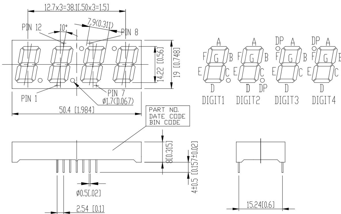
NOTES: All dimensions are in millimeters. Tolerances are ± 0.25 mm (0.01") unless otherwise noted.
