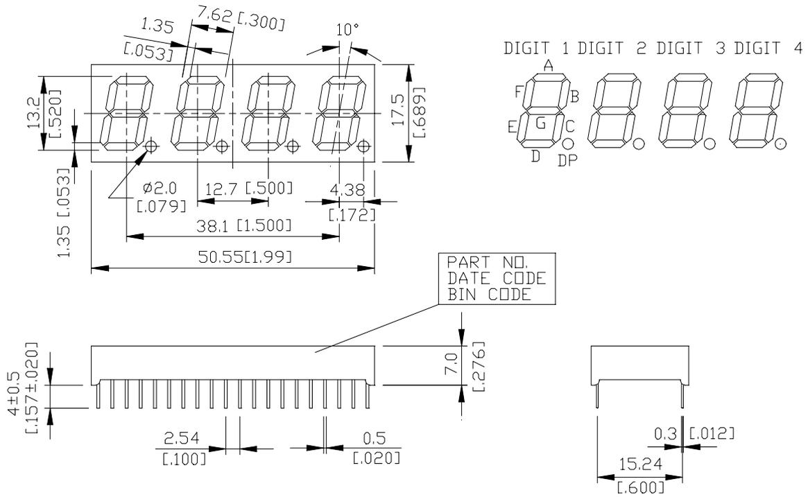
NOTES: All dimensions are in millimeters. Tolerances are ± 0.25 mm (0.01“) unless otherwise noted.
