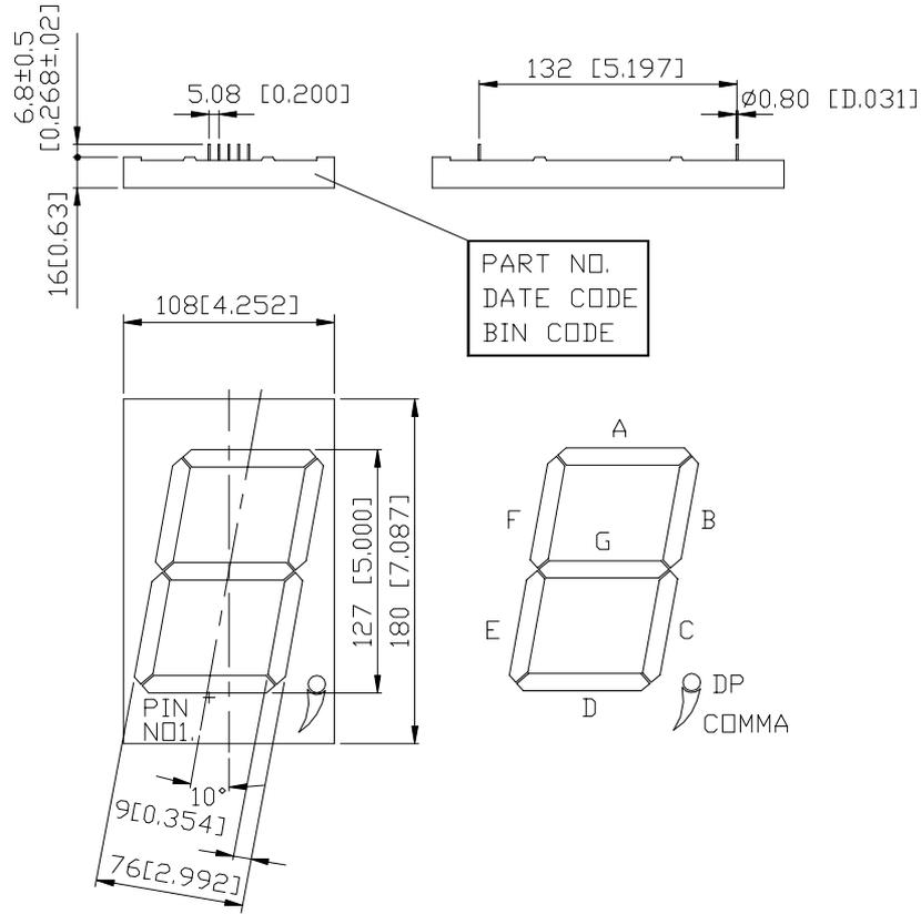
NOTES: All dimensions are in millimeters. Tolerance is ± 0.25-mm (0.01“) unless otherwise noted.
