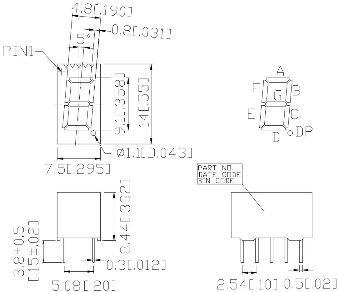
NOTES: All dimensions are in millimeters. Tolerances are ± 0.25-mm (0.01“) unless otherwise noted.
