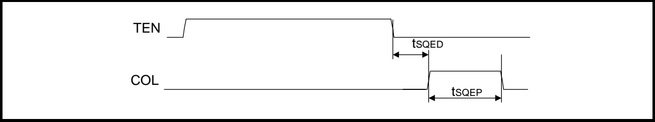
Figure 40: Mode 4 COL/CI Output Timing
