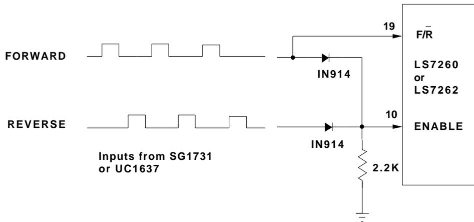
**FIGURE 3. PRECISION CONTROL BRUSHLESS DC MOTOR DRIVE**
