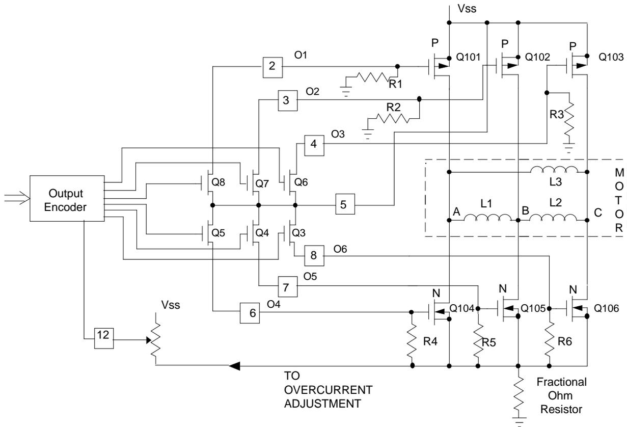
**FIGURE 1. LS7260 THREE PHASE OUTPUT DRIVER CIRCUITRY**
