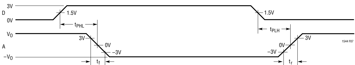
Figure 7. V.10, V.28 Driver Propagation Delays
