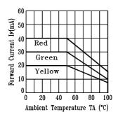
Fig.3 Forward Current Derating Curve
