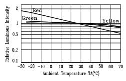
Fig.5 Luminous Intensity vs. Ambient Temperature
