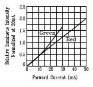
Fig.4 Relative Luminous Intensity vs. Forward Current
