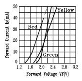
Fig.2 Forward Current vs. Forward Voltage
