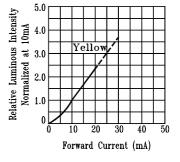
Fig.4 Relative Luminous Intensity vs. Forward Current
